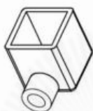
End Cup with a hole at the bottom
